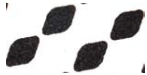
Film with screen dots (Tone value 30%, 100x magnification)
