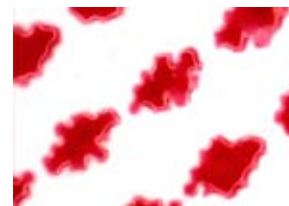
Screen dots printed with standard high-modulus mesh
